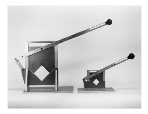
Stoelting's small animal decapitator has hardened and ground surgical stainless steel blades, aluminum base and stainless steel hardware. With its 1 1/2" square maximum blade opening, it is suitable for decapitating rats, mice and other small animals. The decapitator cuts cleanly and quickly through bone and tissue. The base has four holes for bench mounting.
